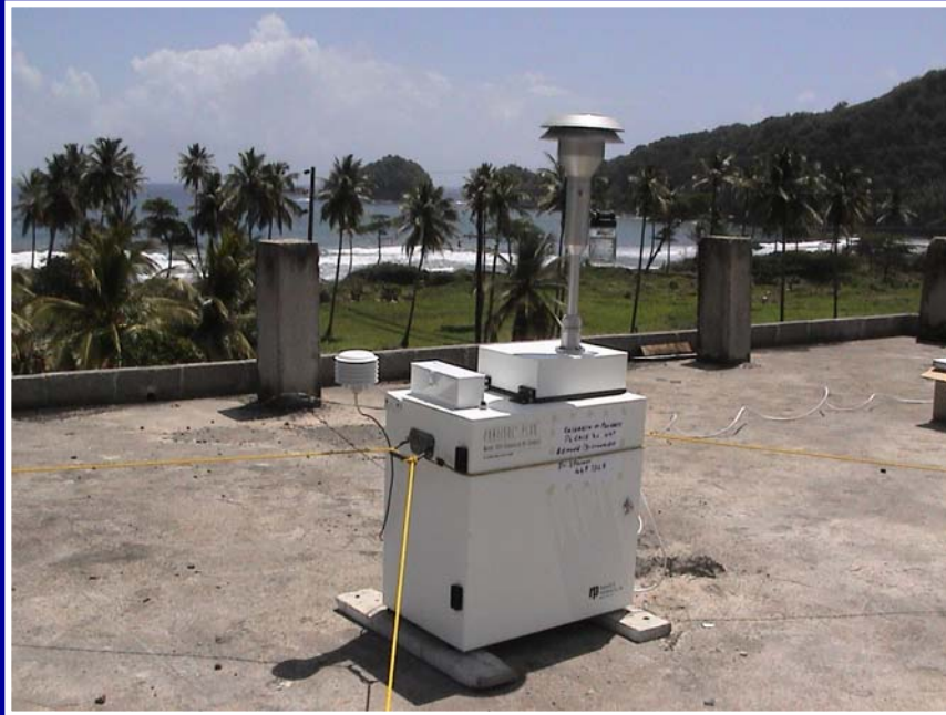
Partisol Plus Model 2025 - Sequential Air Sampler Rupprecht and Patashnick Co., Inc.
